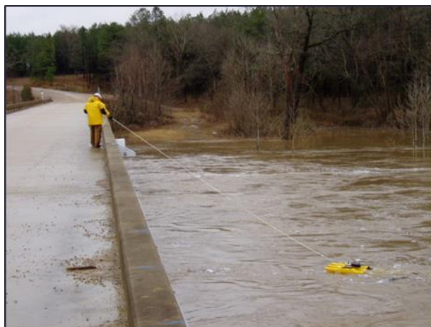
Figure 31 Example of ADCP data collection and transect of velocity profile.
